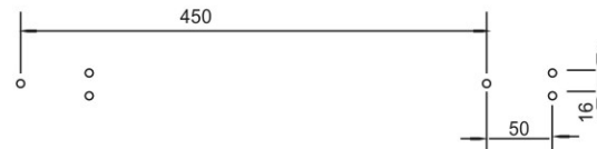
mounting hole for 2000W & 2200W
